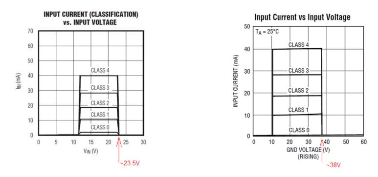
The PD responds with either no/low (couple of mA) current or class current when operated in the undefined region.
