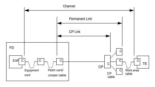
FD = floor distributor; EQP = equipment; C = connection (mated pair);
