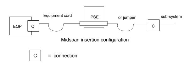
Figure 33–25—Interconnect model, cross-connect model, and midspan insertion configuration
