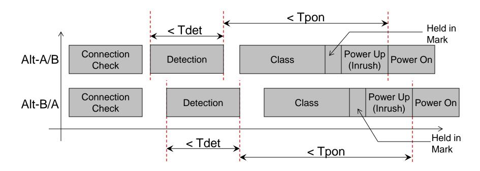
• Each channel can be treated separately, so the timing requirements are the same detection time (Tdet) and power turn on time (Tpon) in the current standard.
