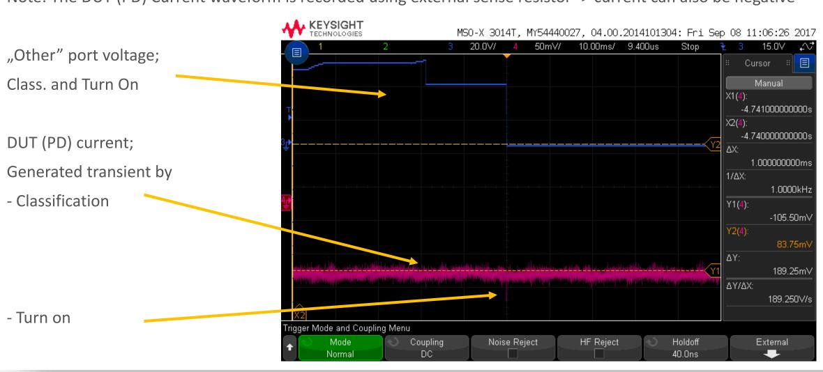
Note: The DUT (PD) Current wavform is recorded using external sense resistor -> current can also be negative
