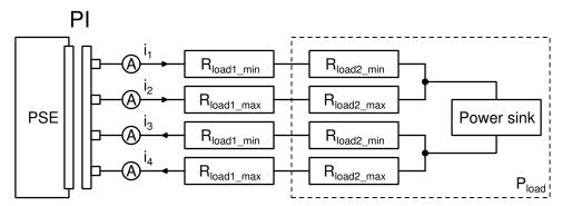
Figure 145-22 - PSE current unbalance verification circuit
