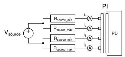
Figure 145-31 — PD current unbalance verification circuit
