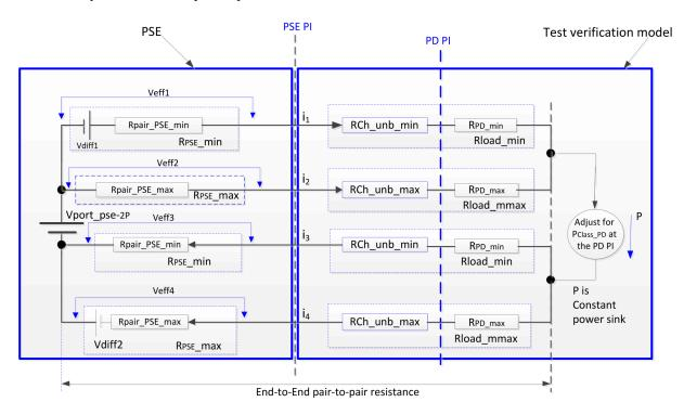
Figure 145A-0a — PD current unbalance verification circuit
