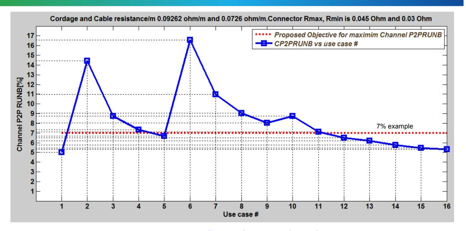
• Lower peaks received with using connector Rdiff=0.015 $\Omega$  instead of 0.02  $\Omega$  compared to previous run.
