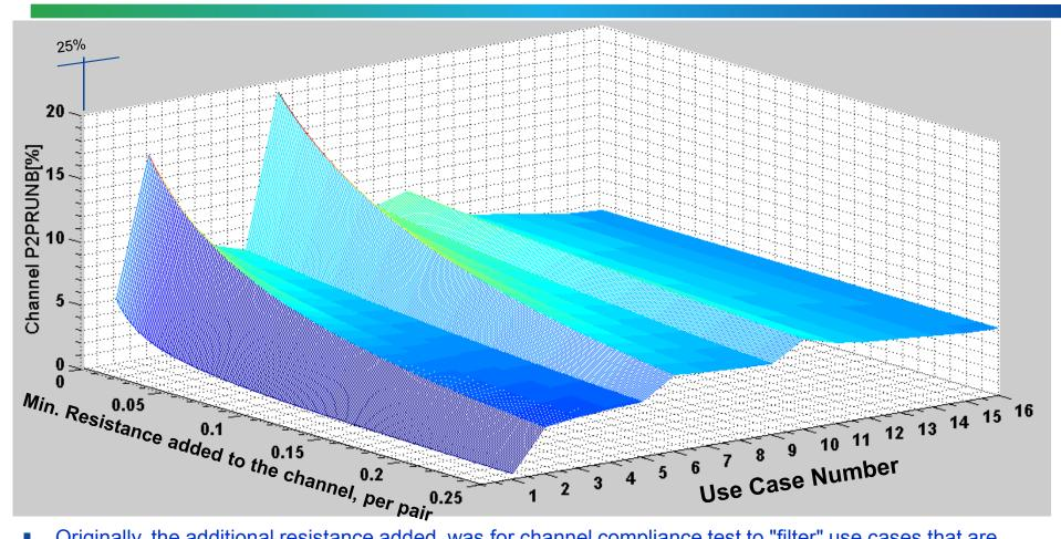
Originally, the additional resistance added, was for channel compliance test to "filter" use cases that are considered as "not typical". Further work showed that the set up may not be required since realistic use case such B is falling into Rdiff=0.1Ω max while the other realistic use case falls within the 7% proposed limit. More over below Rdiff=0.1Ω max, the C\_P2PRUNB is bounded by connectors Runb=25% per the worst case data used in this work
