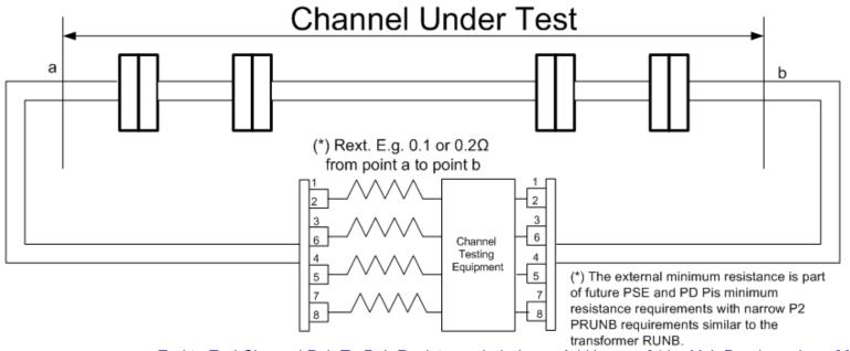
Annex K13 Use case analysis results when adding external minimum resistance requirement per pair for filtering C\_P2PRUNB peaks during: (a) During Channel Compliance test for C\_P2PRUNB. (b) PSE and PD PI).
