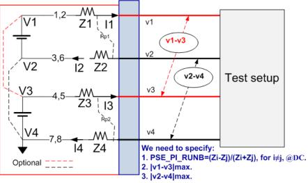
In one typical application: V1=V3, V2=V4=0. As a result, open load voltages: v1-v3 $\rightarrow$  0, v2-v4  $\rightarrow$  0
