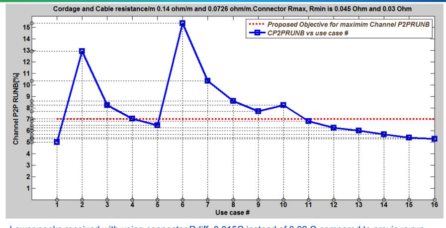
Lower peaks received with using connector Rdiff=0.015Ω instead of 0.02 Ω compared to previous run.
