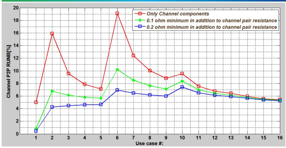
The peaks are filtered when channel is tested with some minimum resistance that exists anyway in PSE and PD PIs. It is equivalent to testing the channel in some minimum system conditions and not just as a channel which is meaningless without minimum requirements from PSE and PD PIs.
