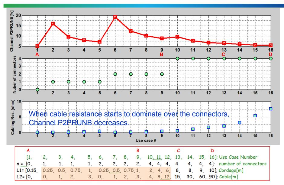
End to End Channel Pair To Pair Resistance Imbalance Ad Hoc rev 011a. Yair Darshan, June 2014
