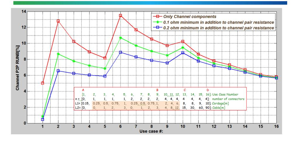
Use case analysis results when adding external minimum resistance requirement per pair for filtering C\_P2PRUNB peaks during: (a) During Channel Compliance test for C\_P2PRUNB. (b) PSE and PD PI).
