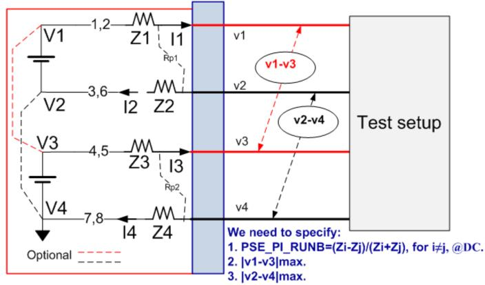
In one typical application: V1=V3, V2=V4=0. As a result, open load voltages: v1-v3 $\rightarrow$  0, v2-v4  $\rightarrow$  0
