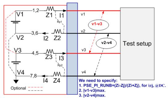
In one typical application: V1=V3, V2=V4=0. As a result, open load voltages: v1-v3→ 0, v2-v4 → 0
