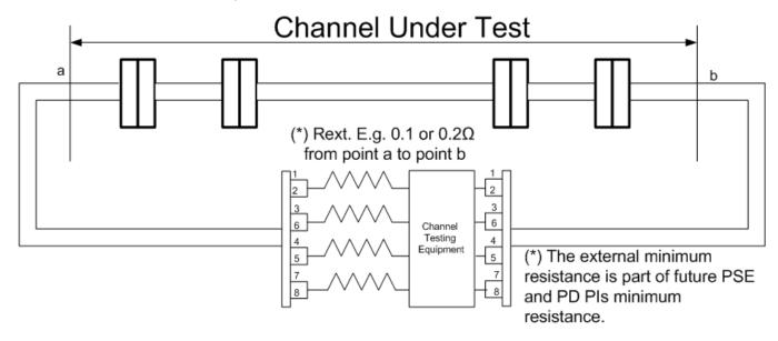
Annex K13 Use case analysis results when adding external minimum resistance requirement per pair for filtering C\_P2PRUNB peaks during: (a) During Channel Compliance test for C\_P2PRUNB. (b) PSE and PD PI).
