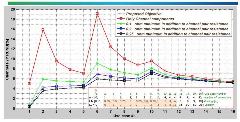
The peaks are filtered when channel is tested with some minimum resistance that exists anyway in PSE and PD PIs. It is equivalent to testing the channel in some minimum system conditions and not just as a channel which is meaningless without minimum requirements from PSE and PD PIs. (C P2PRUNB in 2P system it is irrelevant and in 4P system it is meaningless outside the system)
