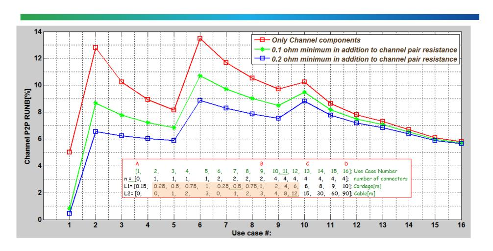
Use case analysis results when adding external minimum resistance requirement per pair for filtering C\_P2PRUNB peaks during: (a) During Channel Compliance test for C\_P2PRUNB. (b) PSE and PD PI).
