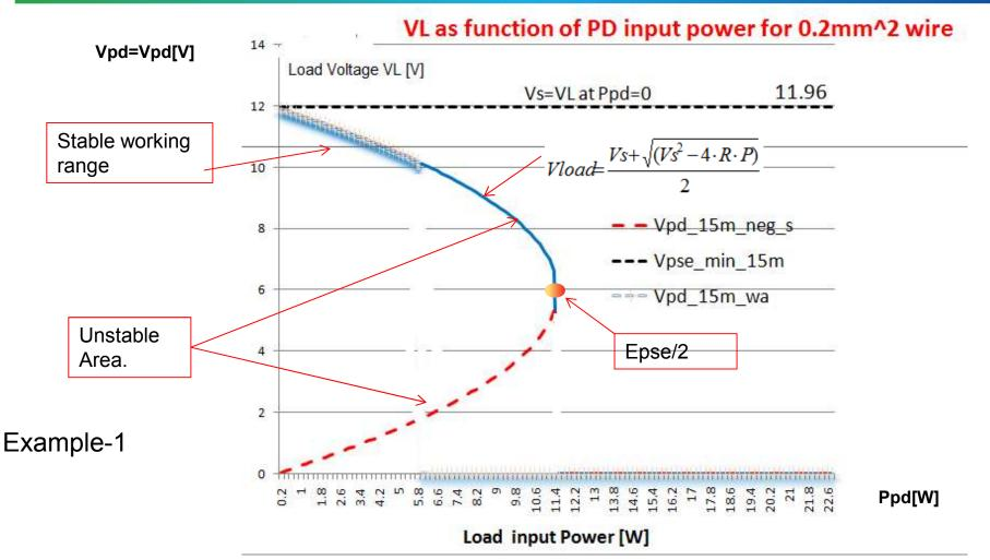
Plot of real system: load voltage vs. load power for 12V source (with 0.4Ω output DC resistance) for supporting 5-6W load
