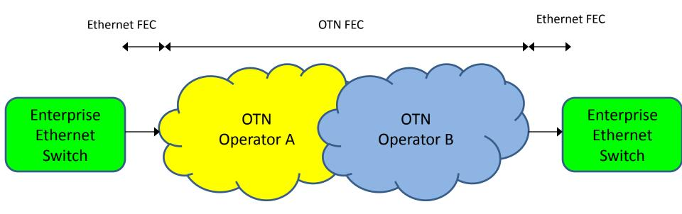
Ethernet FEC must be terminated and regenerated separately for the ingress and egress link
