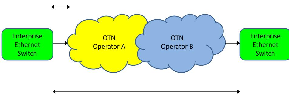
Ethernet FEC is NOT designed to correct all of the errors that may occur across this link
