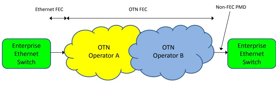
Separating Ethernet FEC for the ingress and egress links allow mix/match of PMD types used at ingress and egress
