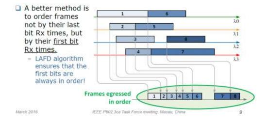
However, the propagation delay of DS channels is different for each channel, due to different fiber lengths and wavelengths. What is worse, this inter-channel skew may change dynamically because of temperature variation or wavelength drift. This inter-channel skew may cause the first bit arrival times to be out of order.
