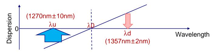
Upstream wavelength ( $\lambda u$ ): 1270±10nm; (TDMA w/ 10G-EPON and 10G-GPON) Downstream wavelength ( $\lambda d$ ): 1357nm±2nm; We have the worst-case DS/US latency differences:
