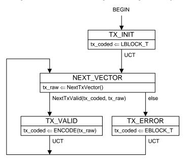
Figure 142- 2 Transmit/Encode State Diagram
