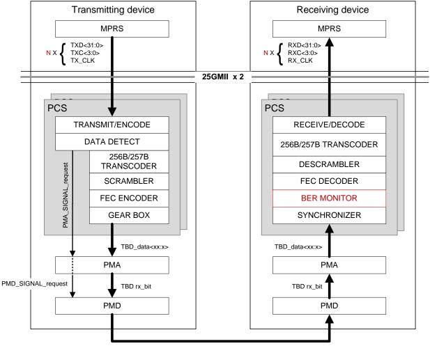
Figure 142- 1 PCS Functional Block Diagram
