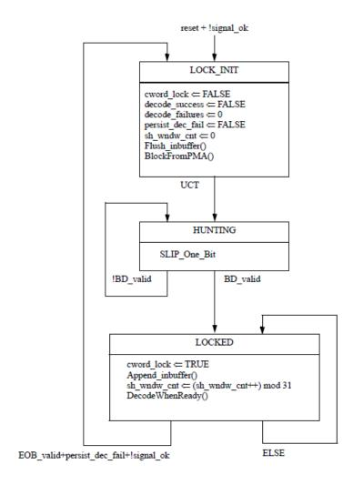
Figure 76-18-OLT Synchronizer state diagram
