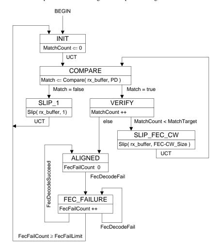
Figure 142-3 ONU Synchronizer state diagram
