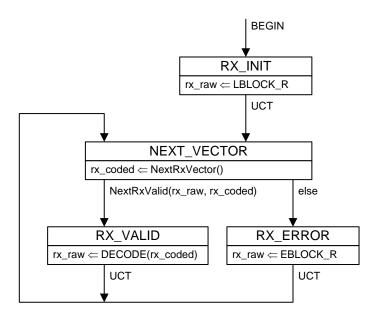
Figure 142- 4 Receive/Decode State Diagram.
