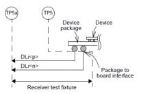
Figure 93-10-Receiver test fixture and test points
