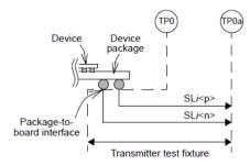
Figure 93-5—Transmitter test fixture and test points
