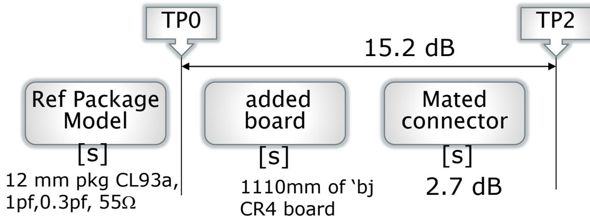
2.5Gb/s Tx Enclosure Set up is physically the same
