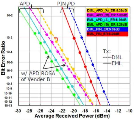
Receiver sensitivities @BER:1e-3 Upper :as Average optical power(AOP) (Lower): as Optical modulation amplitude(OMA)
