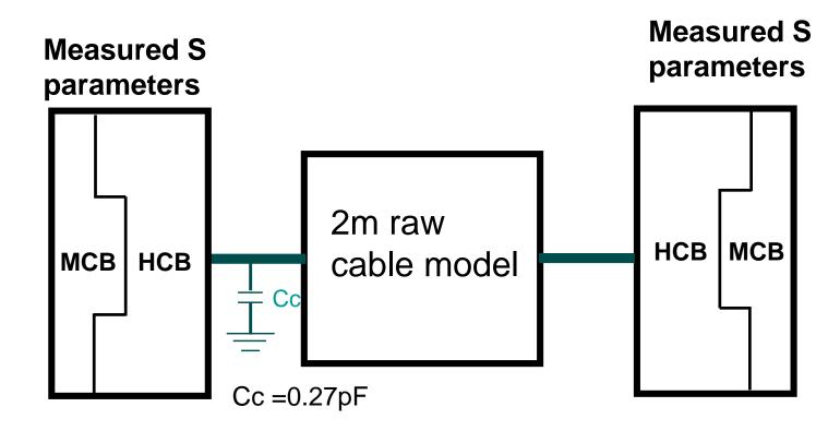
The raw cable model uses the transmission line model in Clause 93A with parameters provided by Rich Mellitz for a 26AWG cable.
