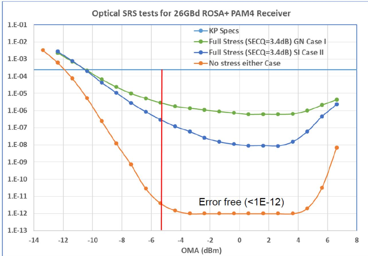
As per [schube 011718 3cd adhoc](#), and according to [chang 3cd 01 1117](#), the top-left transmitter should represent a case in which we are '**Overstressing the receiver** (e.g. if more Gaussian noise is used than the worst-case allowable transmitter) and causing unnecessary yield hit'.
