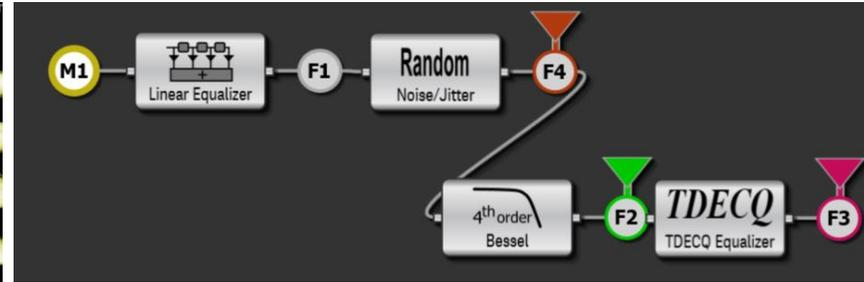
Using Keysight FlexDCA sim tool. Added 5T/2 TX Fir over GoldenEye [shared](#) waveform (kept PRBS13Q for faster processing), random Noise/Jitter block and 4th order BT filter.
