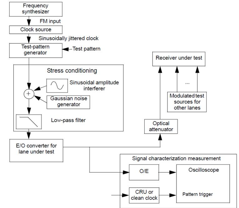
Figure 121-6—Stressed receiver conformance test block diagram
