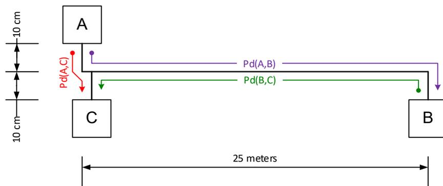
Figure 2 - Worst case maximum propagation delay topology
