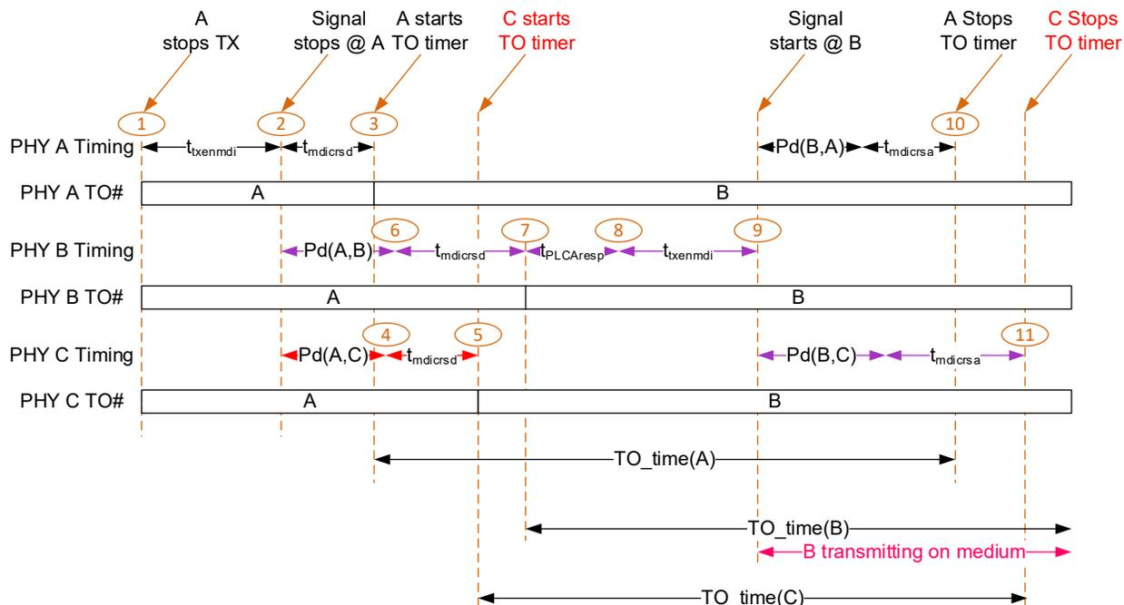
Figure 1 – Timing diagram for computation of transmit opportunity periods along a mixing segment.
