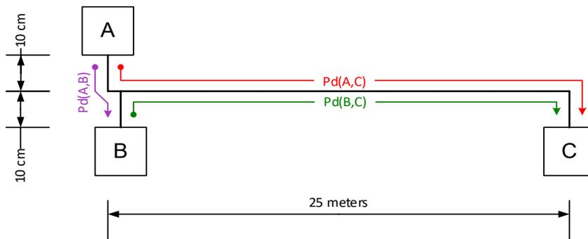
Figure 3 - Worst case maximum propagation delay topology
