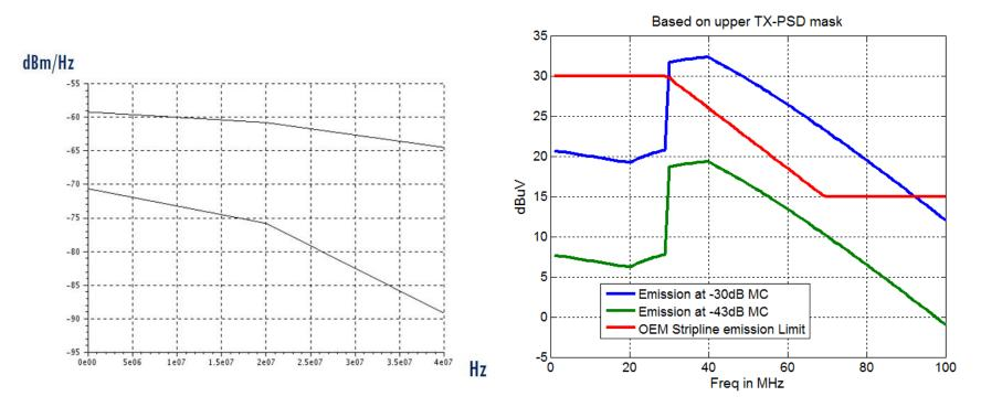
Current TX-PSD mask with -30dB mode conversion (MC) does not meet the emission requirement! Needs cable/connector with better mode conversion
