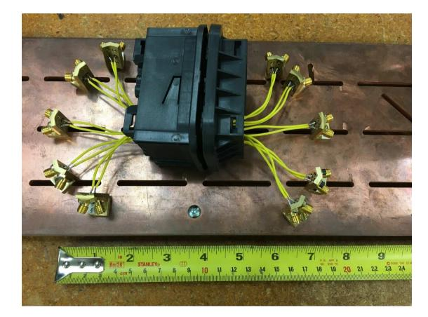
• Termination requires 60-70mm untwist length on each side of the connector
