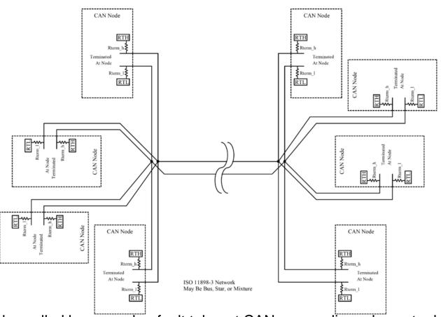
**ISO 11898-3**, also called low speed or fault tolerant CAN, uses a linear bus, star bus or multiple star buses connected by a linear bus and is terminated at each node by a fraction of the overall termination resistance. The overall termination resistance should be about 100  $\Omega$ , but not less than 100  $\Omega$ . Data rate is 40 KB/s up to 125 KB/s
