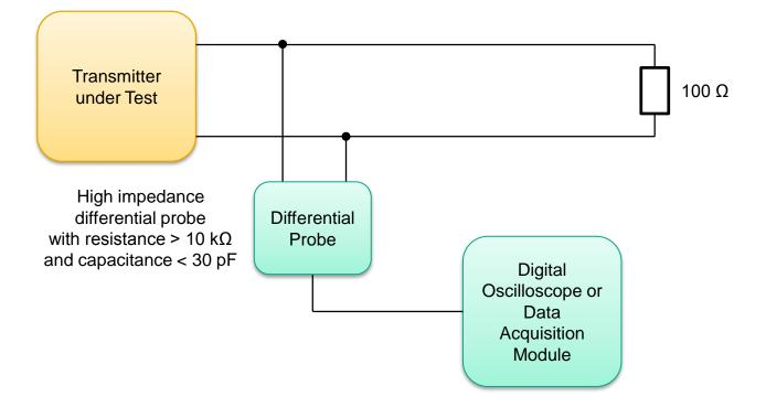
• The test setup is similar to the test setup described in clause 97.5.2.1.
