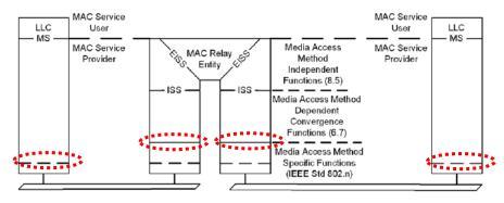
NOTE—The notation "IEEE Std 802.n" in this figure indicates that the specifications for these functions can be found in the relevant standard for the media access method concerned; for example, n would be 3 (IEEE Std 802.3) in the case of Ethernet.
