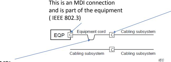
This is a cabling interface connection and is part of the cabling (ISO/IEC WG33)
