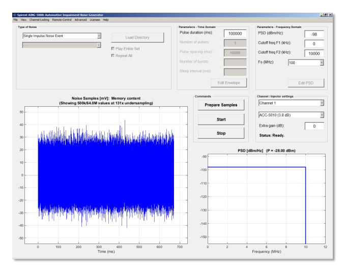
• AWGN noise with -98 dBm/Hz and a bandwidth of 10 MHz does not cause any bit errors within a run time of 100 s.
