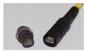
Prototype M8 style, plug overmolded and straight PCB THT jack with housing
