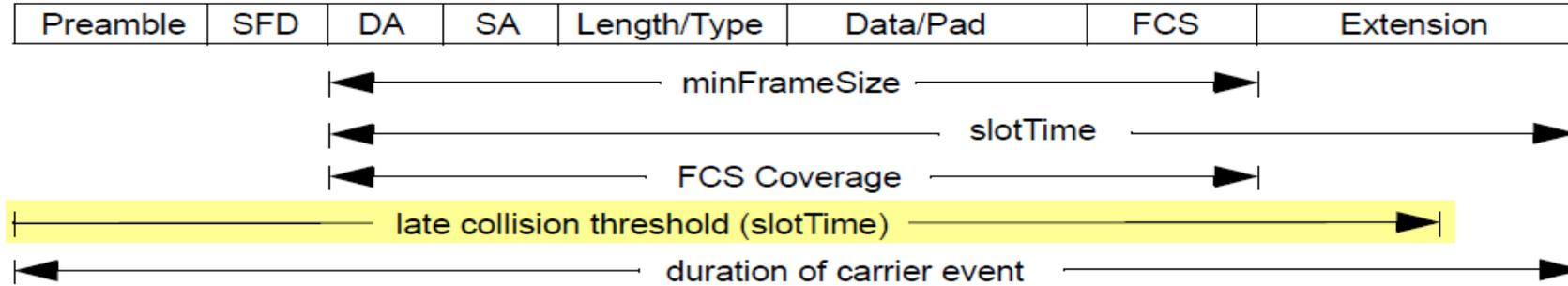
Figure 4-5—Frame with carrier extension
