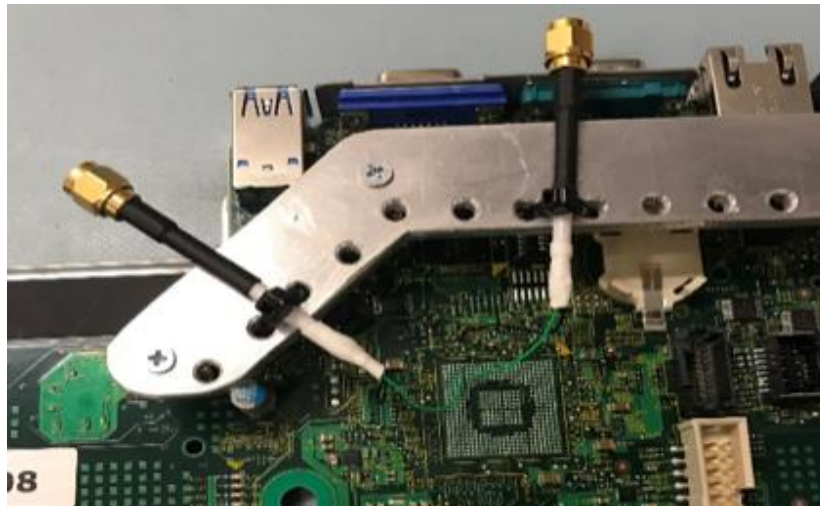
Board Management Controller (Bus Master)
