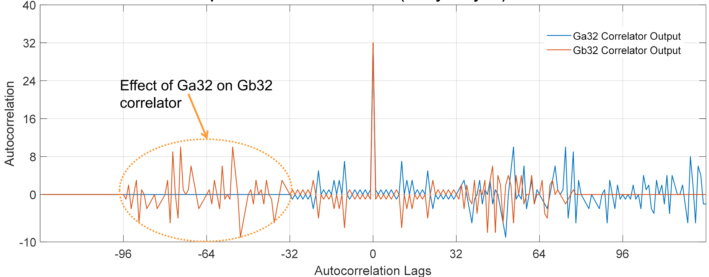
Correlation of Proposed Preamble with Ga32 (Delayed by 64) and Gb32 Correlators
