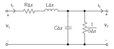
Standard analysis shows that its behaviour is governed by Characteristic Impedance, Z<sub>0</sub>, and Propagation Constant ,γ, with the ABCD matrix being:
