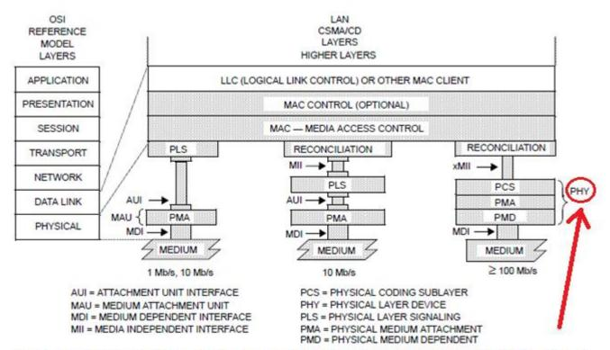
NOTE—In this figure, the xMII is used as a generic term for the Media Independent Interfaces for implementations of 100 Mb/s and above. For example: for 100 Mb/s implementations this interface is called MII; for 1 Gb/s implementations it is called XGMII; etc.
