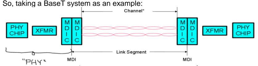
So here the PHY includes the transceiver chip ('PHY chip') plus the transformer ('XFMR') plus the PCB traces etc up to the MDI interface
