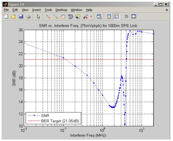
Fail to meet SNR target for BER of 1e-9 for interferer frequency from ~100kHz -> ~4MHz
