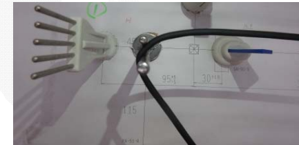
Figure 3: Bending on Jig board
