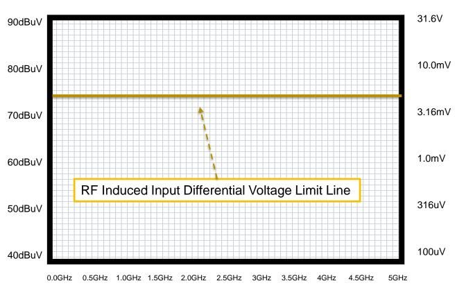
The limit line used for the differential voltage magnitude at the PHY input induced by the RF fields coupled to the STP cable, which was used for the analysis
