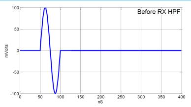
One cycle of a 20MHz sinusoidal signal with magnitude of 100mV is suggested for system analysis of transient noises.
