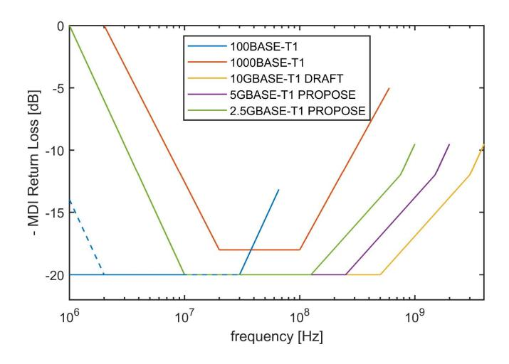
▶ 2.5GBASE-T1 >2x tighter than 1GBASE-T1, so sufficient
