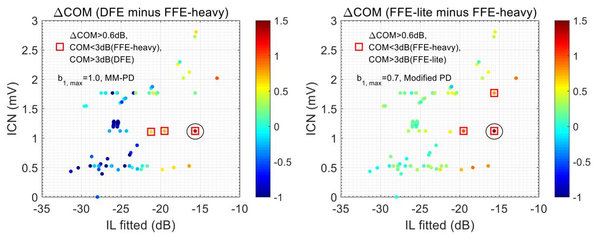
• DFE may pass the same channels as FFE-lite with large margins which can not be supported by FFE-heavy receivers. This is due to the long DFE that exists in both receivers.
