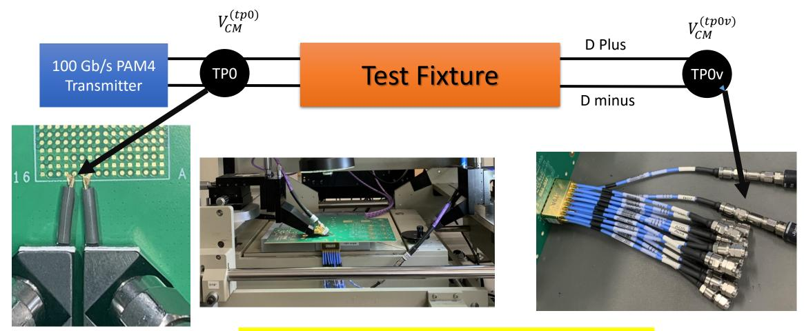
At some low enough frequency the common mode voltage at TPO and TPOv are approximately the same.
