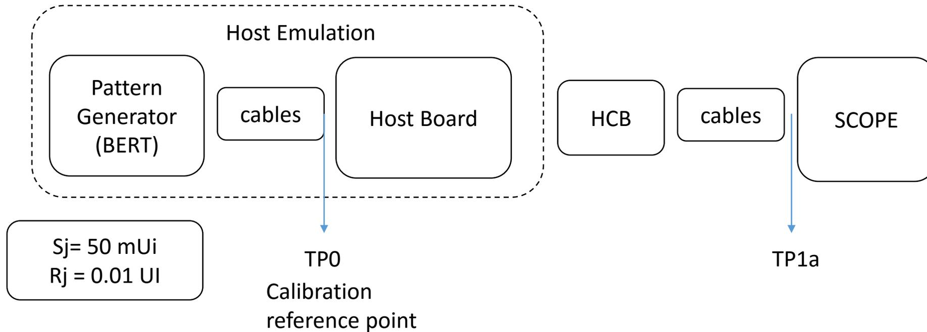
Measure  $J_{4u}$  and  $J_{RMS}$  → Compute  $A_{dd}$  and  $\sigma_{rms}$
