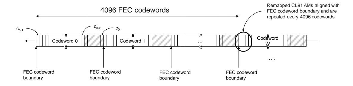
The CL91 Alignment Markers are aligned with RS(544, 514) FEC boundary. As long as the FEC boundary is founded by the self-synchronization algorithm, the FECLs can be easily recovered.
