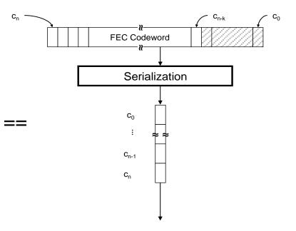
"Keep all the FECLs in order and use 4:1 symbol mux." is equivalent to direct "symbol mapping" from the FEC codeword to 1 PMD lane.
