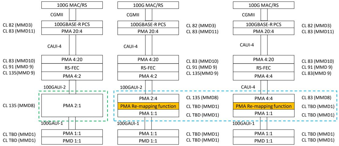
PMAs without re-mapping The same as C2M Add an optional PMA remapping function for difficult channels of multitap DFE.
