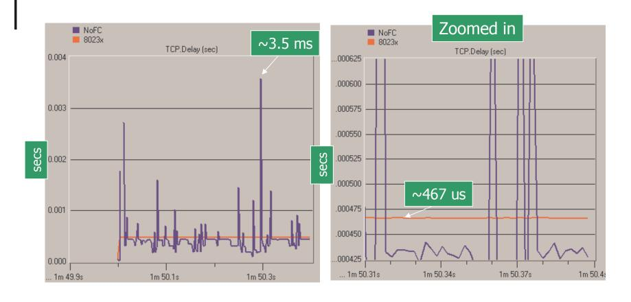
802.3x can provide significantly lower jitter
