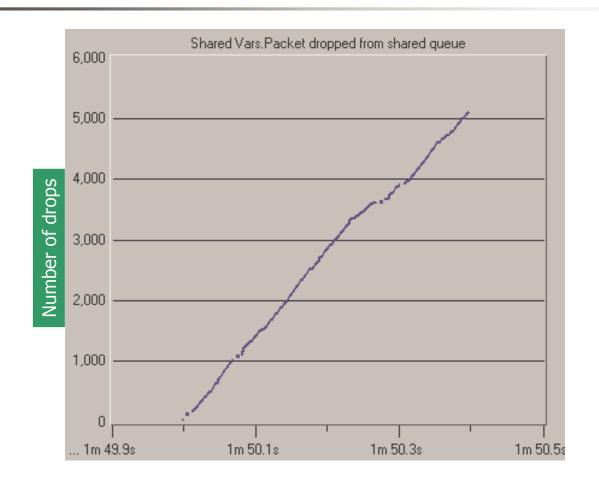
Flow Control can eliminate packet drops
