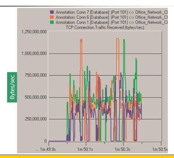
With no Flow Control, all the sources continuously compete for BW Poor sharing with non-deterministic and uneven distribution between sources
