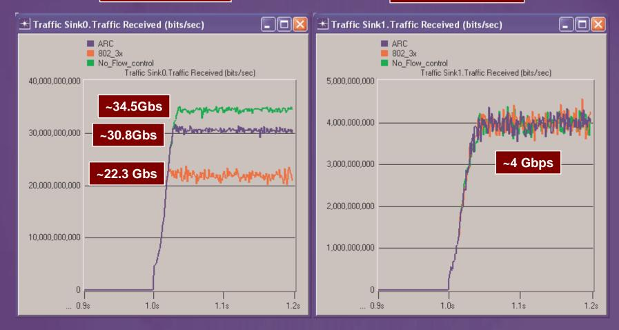
Adaptive Rate Control Provides better throughput than 802.3x.
