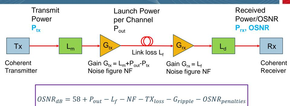
$$TX_{loss} = 10Log\left(1 + \frac{10^{-\frac{L_f}{10}} 10^{\frac{P_{out}}{10}}}{10^{-\frac{L_m}{10}} 10^{\frac{P_{tx}}{10}}}\right)$$
