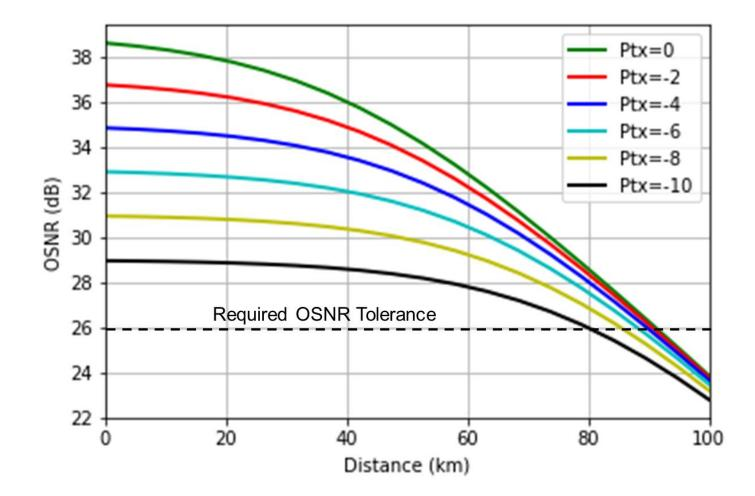
Note OIF ZR specs. are min. Tx power = -10 dBm, and required OSNR = 26 dB
