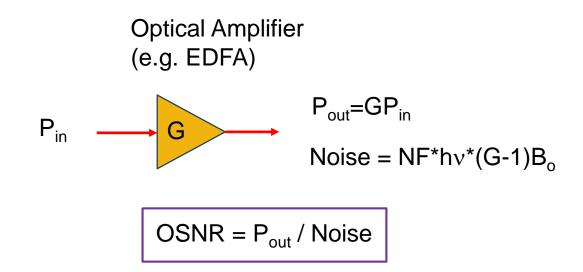
OSNR = ratio of signal power to optical noise
