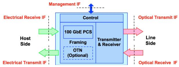
Figure <u>1040 – Dual Optical Interface</u> Transceiver Optical, Electrical and Management Interfaces
