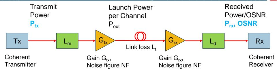
$$OSNR_{dB} = 58 + P_{out} - L_f - NF - TX_{loss} - G_{ripple} - OSNR_{penalties}$$
