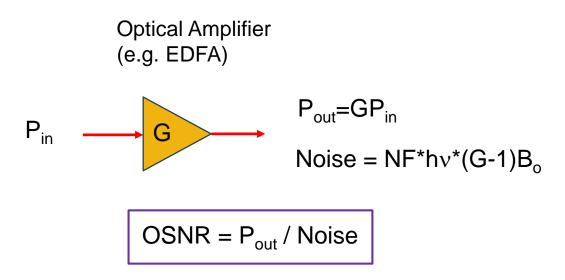
OSNR = ratio of signal power to optical noise
