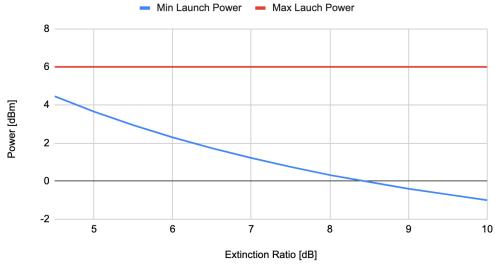
Figure 4 - Acceptable ONU Launch Power at 2.5Gb/s
