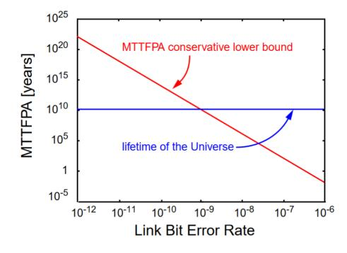
While this may seem like overkill, users want a low rate of false packet acceptance in a network containing a large number of Ethernet links and also it is desirable that the MTTFPA remains reasonable when the link BER is worse than the specification level.
