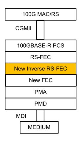
The optional Inverse RS-FEC sublayer "unwinds" the RS-FEC (Clause 91) sublayer, allowing a new FEC sublayer to be inserted further down the stack
