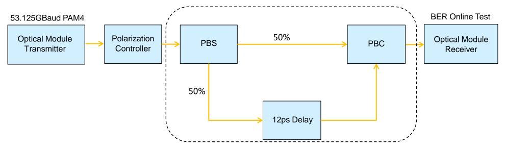
This module can only introduce 12ps of time delay by the components with fixed size .
