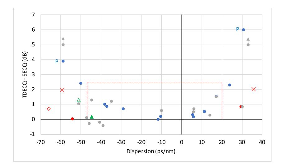
johnson\_optx\_01\_0319 un-optimised johnson\_optx\_01\_0319 optimised yu\_optx\_01a\_0319 yu\_optx\_01a\_0319 predicted Ρ lewis\_cu\_adhoc\_041719 schube\_3cu\_01\_0519 Si Ph (CD pen) X mazzini\_3cu\_adhoc\_082119 Si Ph 100G Lambda MSA 100G Lambda MSA excessive -47 to 20 ps/nm with 2.5 dB penalty
