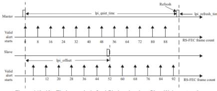
Figure 149–13—Timing periods for LPI signals when Slow Wake not active
